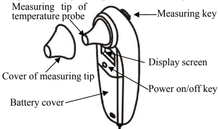
Figure 2.7A the infrared temperature probe
