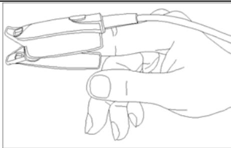
Figure 2.6 demonstration for SpO<sub>2</sub> probe
